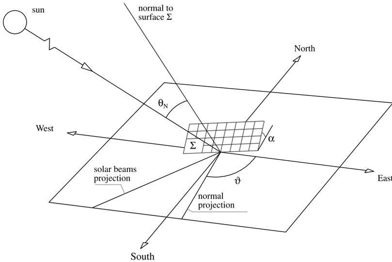
Figure 1 Solar irradiance on a tilted surface
